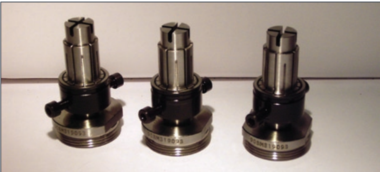
Special mandrel assemblies used in aircraft assembly.
